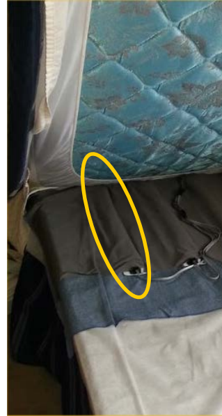
Hydraulic bed sensor under the mattress captures quantitative pulse, respiration & restlessness
